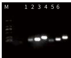
Figure 1: Purified DNA fragments from gel Lane 1-3: Before purification of 80 bp, 120bp, 200bp DNA Lane 4-6: After purification of 80 bp, 120bp, 200bp DNA Gel DNA fragments Purified using CommaPrep™ NP10, elution volumn was 50 µL, sample volumn was 6 µL for AGE.
